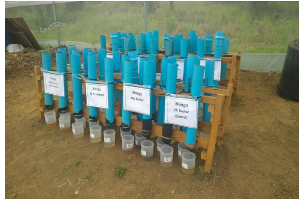
Figure 2. Leaching experiment on benchmark soils of Zambia
