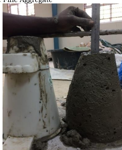
Figure 003: Measuring the Slump Height of Plastic Modified Concrete
