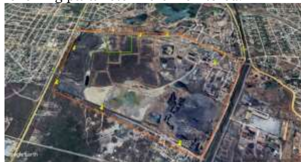
Figure 8: Description of the Monitoring Borehole Locations indicated in yellow as ground-water (GW)
